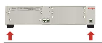
4. For desktop mount. Install feet using plastic push rivets.
