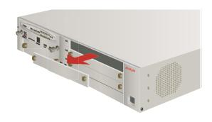
1. To install a media module, first remove the upper right blank faceplate.
