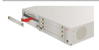
1. From the front of the G700 Media Gateway, remove the blank faceplate from slot V1.
