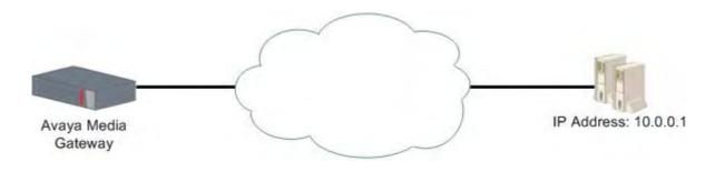
1. The first step is to configure an RTR which tracks a remote device. In this case, RTR 5 is configured to track the device at IP address 10.0.0.1. For example:
