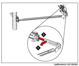
5. Pull out the mounting bracket pin (7) and slide the mounting bracket (8) into the slide rail onto which you are installing the cable-management arm. See the following figure.
