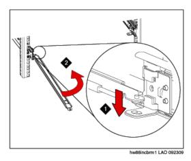
2. Install the L-shaped cable-management stop bracket (3) on the unattached end of the support arm. See the following figure
