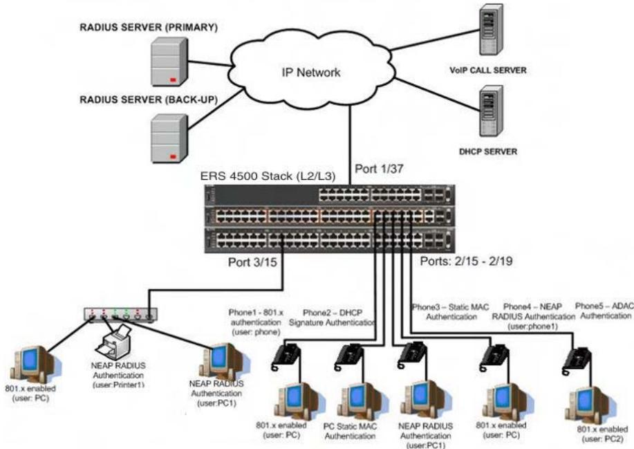
**Figure 33: MHMA authentication mode (Multihost MultiVLAN option disabled) with or without additional RADIUS attributes**
