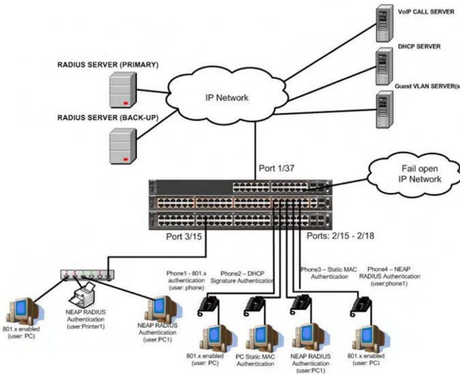
**Figure 37: MHMA authentication mode with Guest VLAN and Fail Open VLAN (Multihost MultiVLAN option disabled) with or without additional RADIUS attributes**
