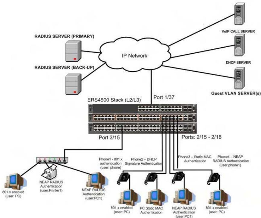
**Figure 35: MHMA authentication mode with Guest VLAN (Multihost MultiVLAN option disabled) with or without additional RADIUS attributes**
