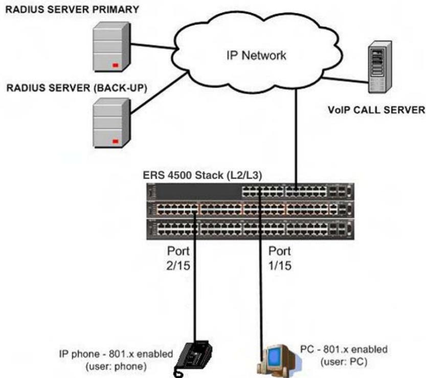
**Figure 27: SHSA authentication mode with or without RADIUS additional attributes with or without Multihost MultiVLAN**
