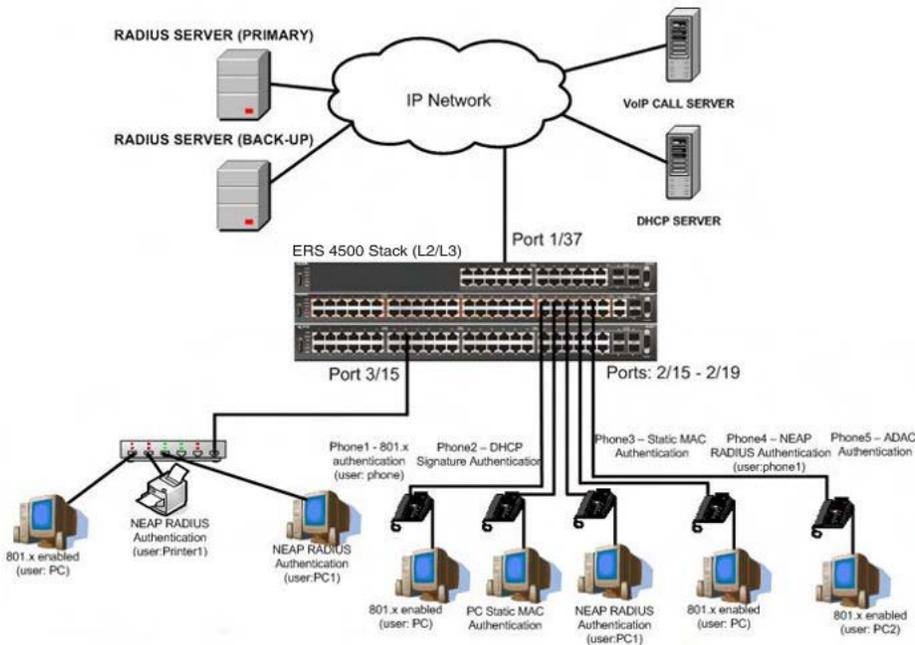
**Figure 34: MHMA authentication mode (Multihost MultiVLAN option enabled) with or without additional RADIUS attributes**
