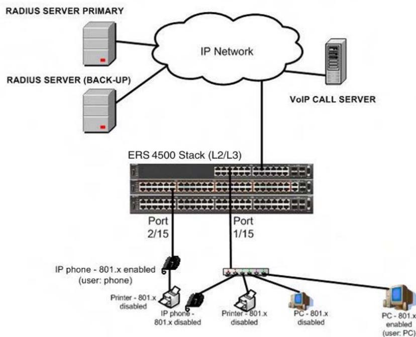
**Figure 30: MDSA authentication mode (with or without RADIUS VLAN and with or without Multihost MultiVLAN enabled)**
