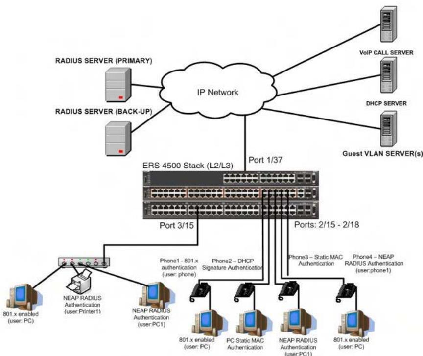
**Figure 36: MHMA authentication mode with Guest VLAN (Multihost MultiVLAN option enabled) with or without additional RADIUS attributes**
