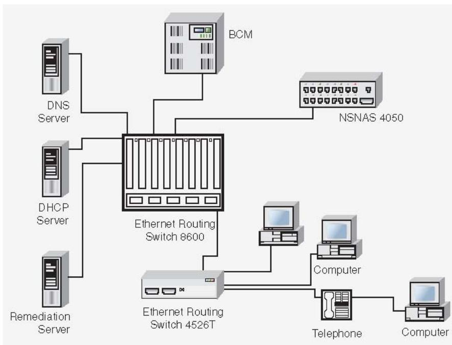
**Figure 4: Network access device-Layer 2 mode**
