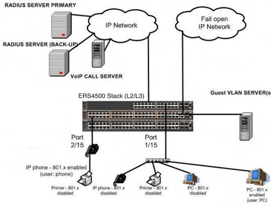
**Figure 32: MSA authentication mode (Guest VLAN and Fail Open VLAN options enabled) with or without Radius additional attributes and with or without Multihost MultiVLAN option**
