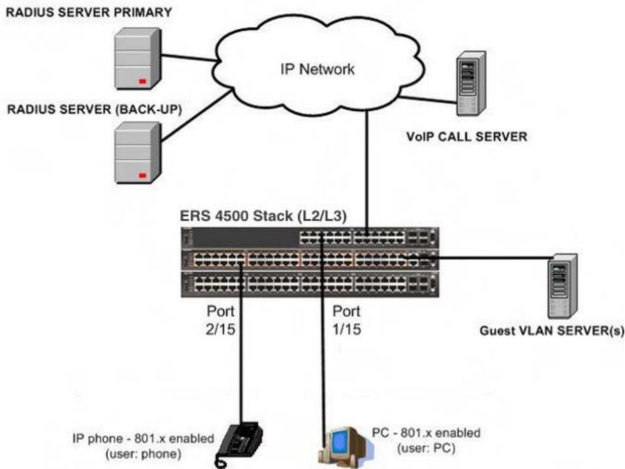
**Figure 28: SHSA authentication mode (with Guest VLAN enabled) with or without RADIUS additional attributes, with or without Multihost MultiVLAN**
