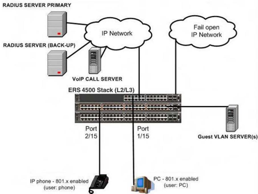
**Figure 29: SHSA authentication mode (with Guest VLAN and Fail Open VLAN enabled) with or without RADIUS additional attributes with or without Multihost MultiVLAN**
