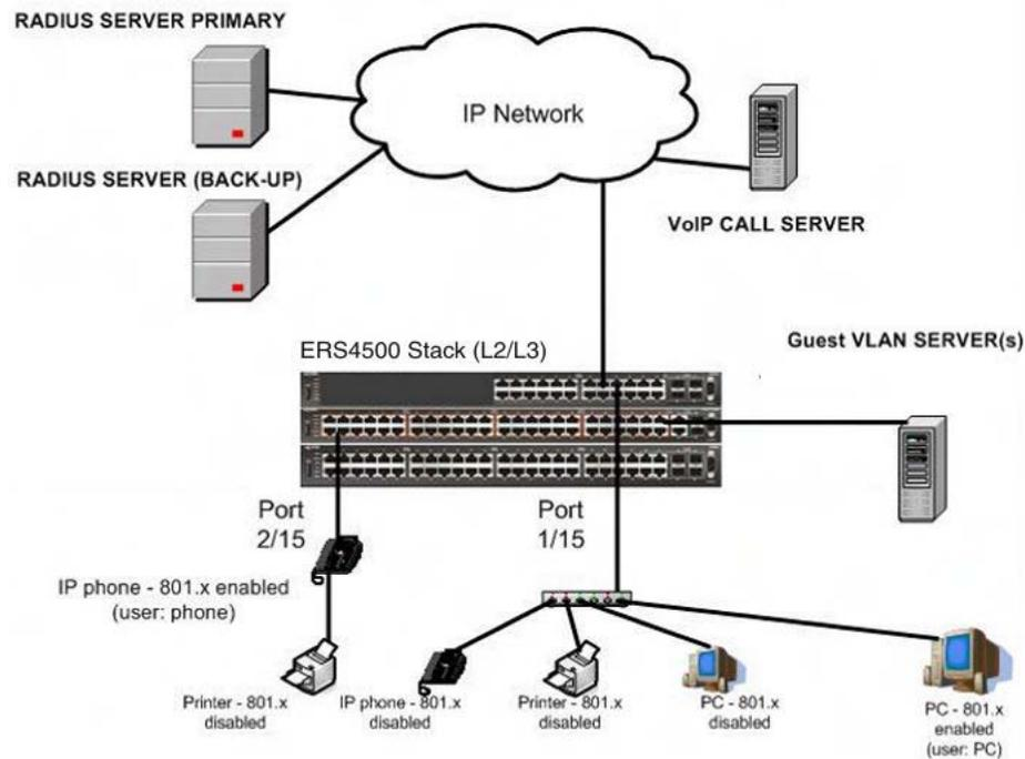
**Figure 31: MHTA authentication mode (Guest VLAN option enabled) with or without RADIUS additional attributes with or without Multihost MultiVLAN**
