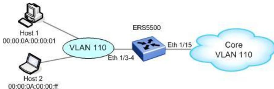
Figure 5: L2 Classification Based on MAC Address Example
