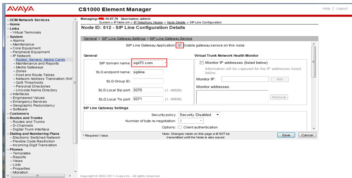
**Figure 7: Adding a new IP Telephony Node (cont)**
