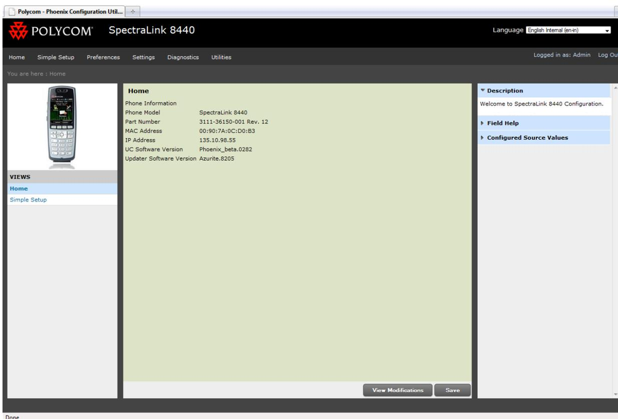
**Figure 21: Home page of Polycom SpectraLink 8440 telephone**
