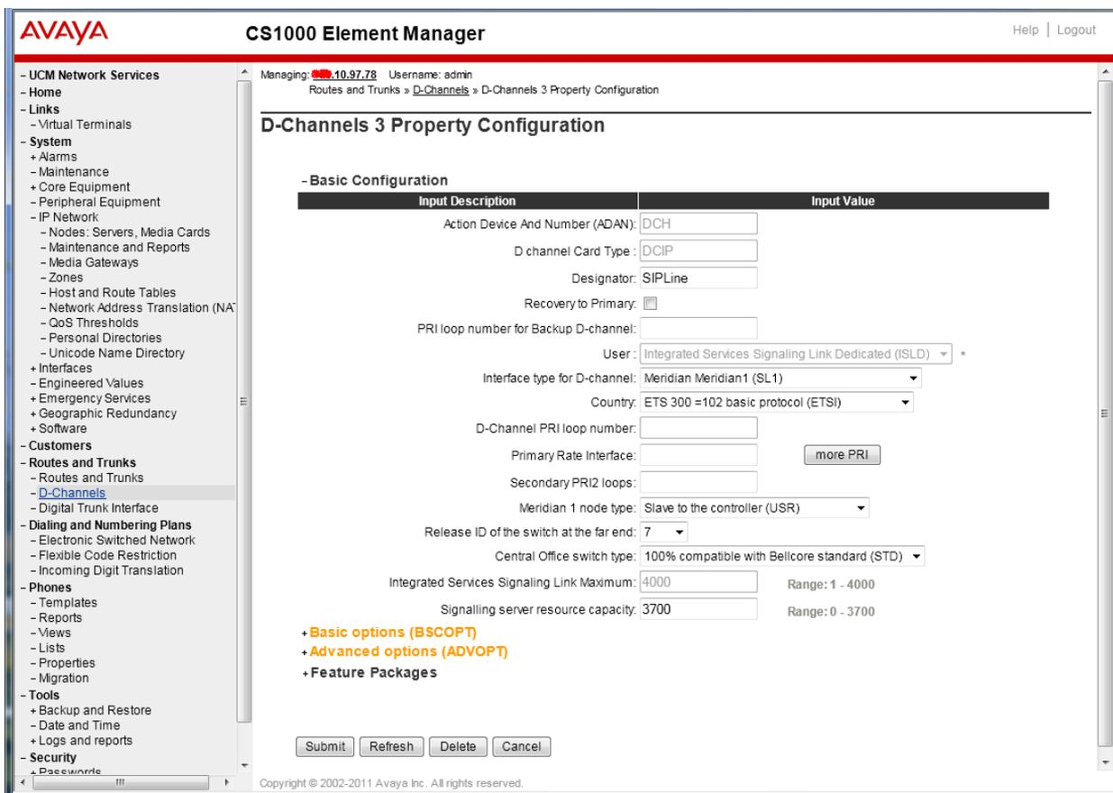
**Figure 12: SIP Line D-Channel Property Configuration**
