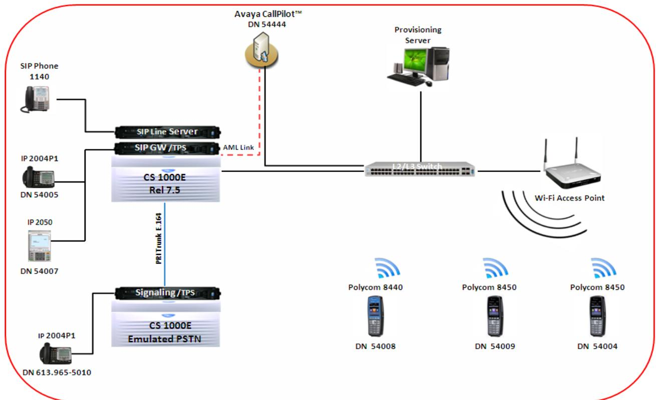
**Figure 1: Network Configuration Diagram**
