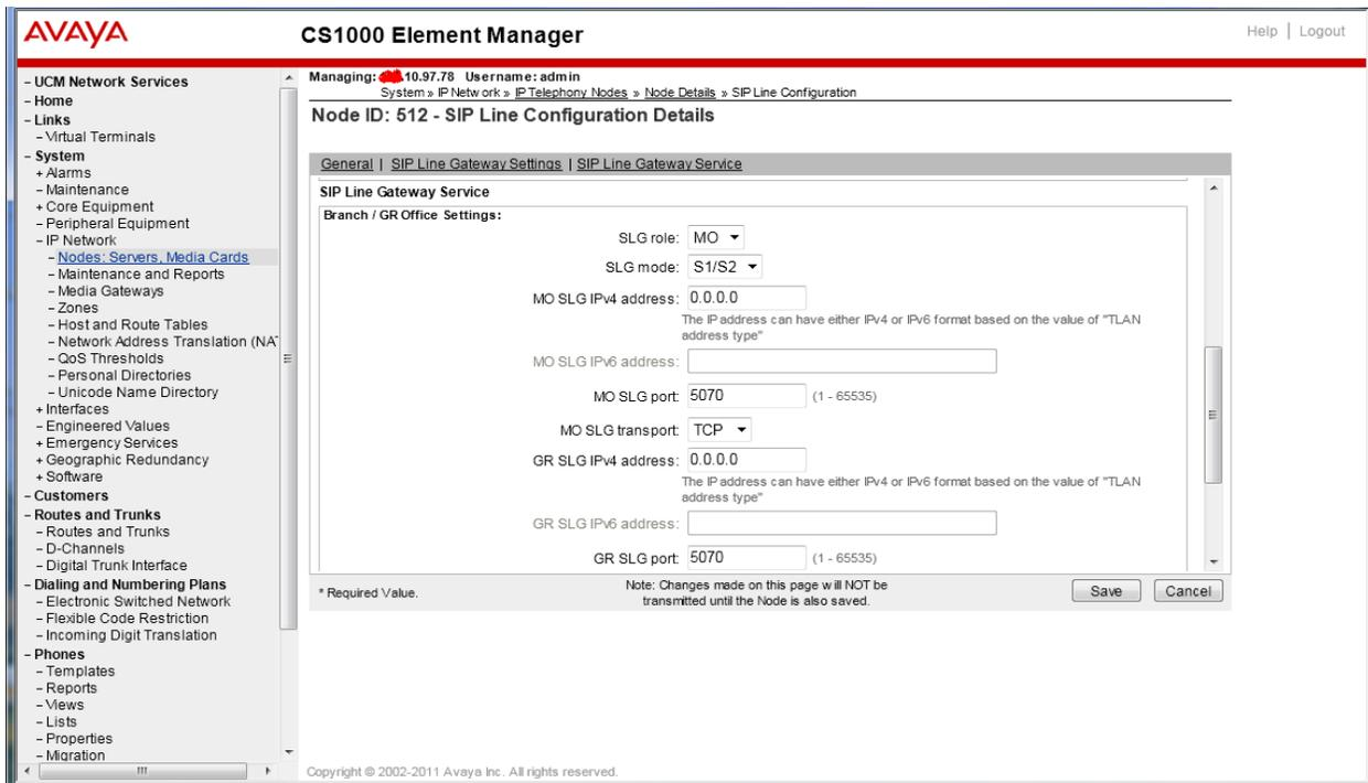
**Figure 8: Adding a new IP Telephony Node (cont)**
