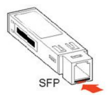
The following figure shows the wrap-around latch-type extraction mechanism. To remove the device, push the collar towards the module.
