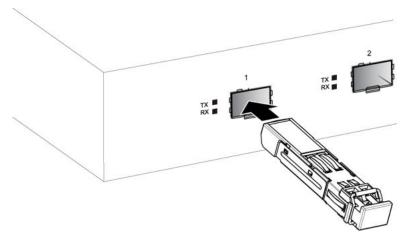
4. Remove the dust cover from the optical bore and insert the fiber optic connector.
