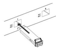
4. Remove the dust cover from the XFP optical bores and insert the fiber optic cable.
