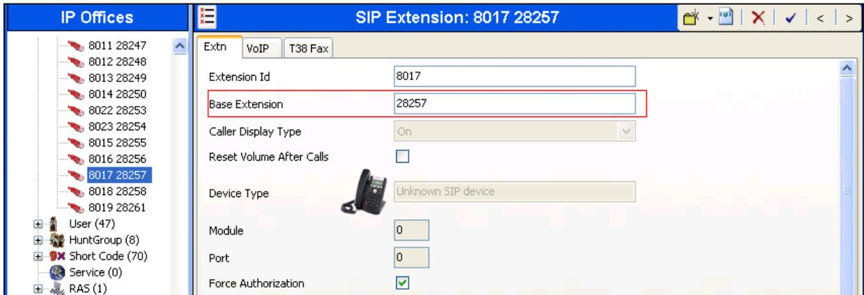
Select the **VoIP** tab, and retain the default values in all fields. Repeat this section to add another new SIP extension for a second Yealink VP530 SIP phone. During the compliance test, extensions **28257** and **28258** were created for two Yealink VP530 SIP phones.
