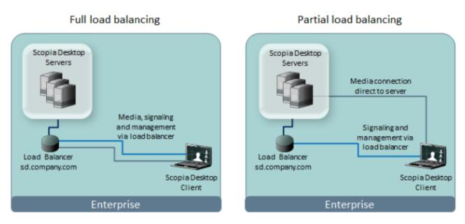
Figure 92: Media can either bypass or travel via the load balancer
