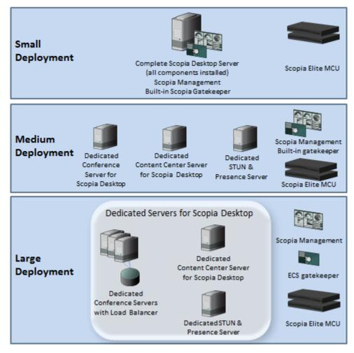
Figure 3: Typical Scopia Desktop Server setups based on size of deployment
