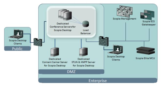
Figure 11: Typical load balanced Scopia Desktop deployment
