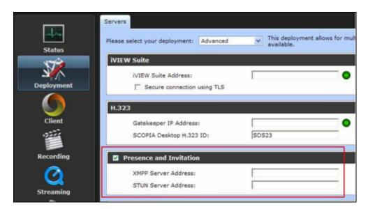
Figure 69: Connecting the Scopia Desktop Server to presence (XMPP) and STUN servers
