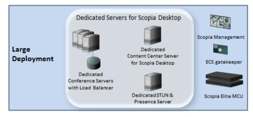
Figure 8: Typical large deployment
