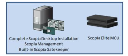
Figure 4: Typical small deployment of Scopia Desktop Server
