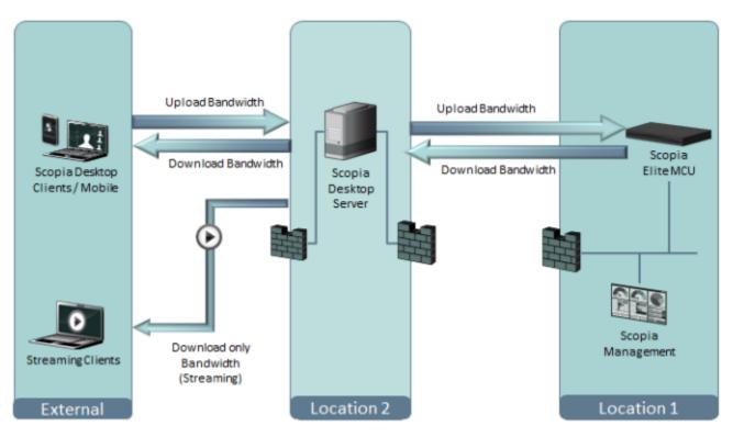
Figure 21: Fragmented distributed deployment requires more external bandwidth
