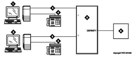
Figure 11: DCP Personal Computer interface configuration (Group 1)
