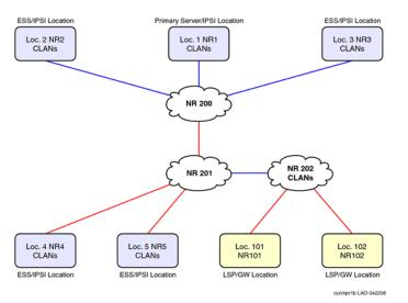
Figure 2: Pre-CM5.1 workaround for unwanted C-LANs
