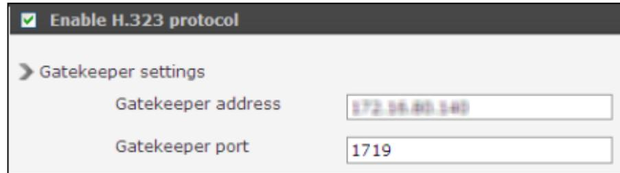
**Figure 32: H.323 Protocol section of the Protocols tab**
