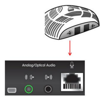
Figure 20: Connecting the Microphone Pods to the XT Codec Unit
