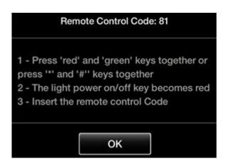
Figure 36: Setting the code on the XT Remote Control Unit
