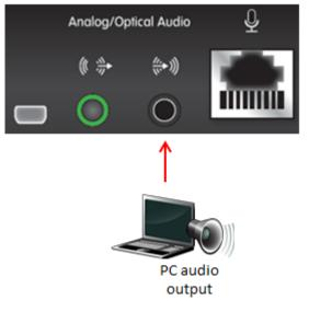
Figure 17: Connecting the computer's audio to the XT Codec Unit
