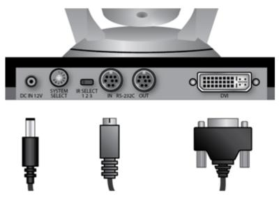
Figure 25: Connecting cables to the back of the camera
