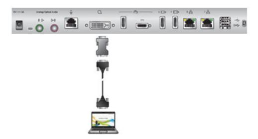
Figure 8: Connecting a computer to Scopia XT Series
