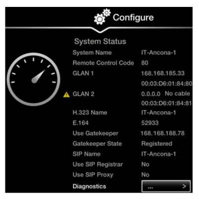
Figure 77: Viewing system network information
