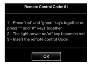
Figure 14: Setting the code on the XT Remote Control Unit
