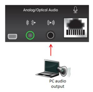
Figure 9: Connecting the computer's audio to the XT Codec Unit
