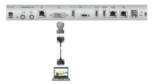
Figure 47: Connecting a computer to Scopia XT Series
