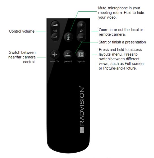
Figure 10: The new XT Remote Control Unit
