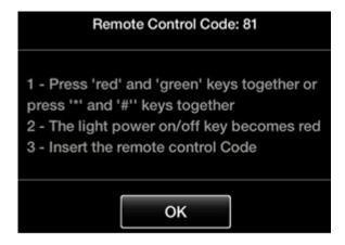
Figure 12: Setting the code on the XT Remote Control Unit
