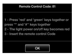
Figure 49: Setting the code on the XT Remote Control Unit
