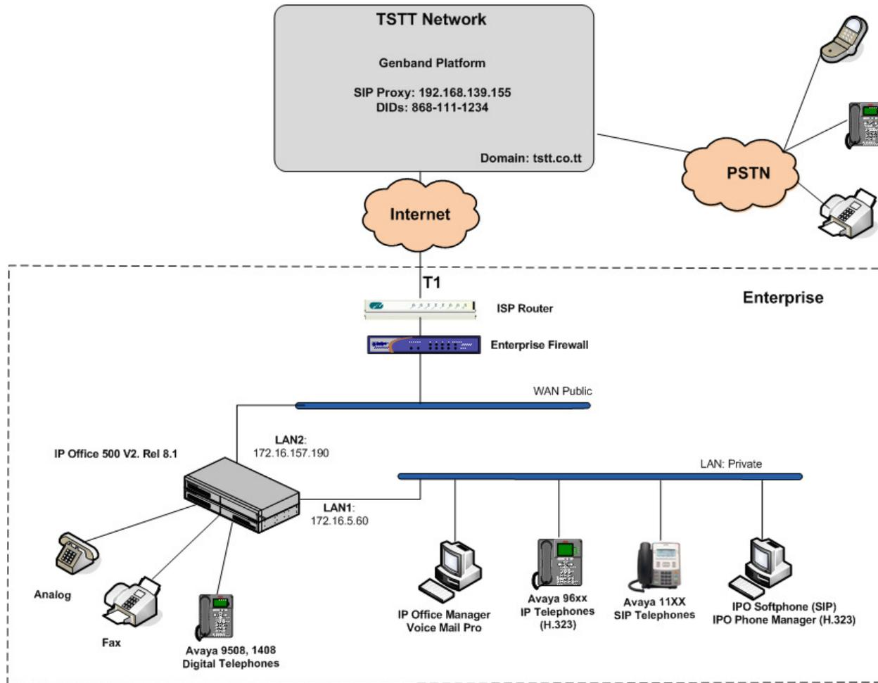
Figure 1: Test Configuration
