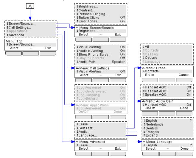
The following options are not used with IP Office and are not included in this documentation; **Applications**, **Log-Answered**, **Log-Outgoing**, **Log-Bridged**, **Erase Contacts**, **Erase Call Log** and **Stay in Contacts**
