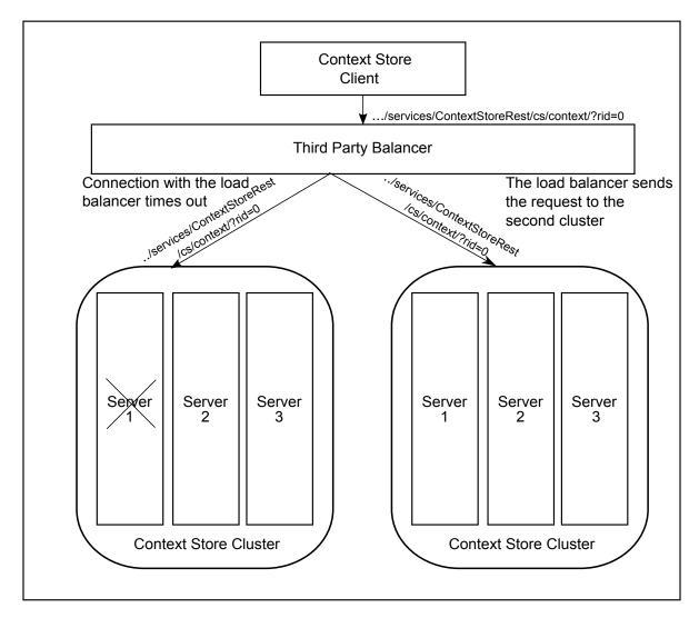
• Either of the Avaya Breeze<sup>™</sup> servers and the other server of a Context Store cluster is unavailable, the remaining server detects the failure and returns a status code of 500. Upon receiving the failure information from the remaining server, the load balancer routes all requests to the other cluster in the geo redundant system.
