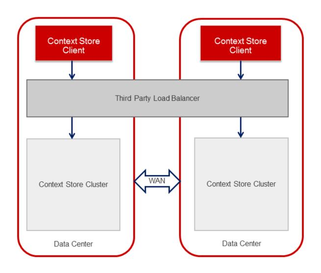
Two Context Store clusters are deployed at two different data centers. All requests to Context Store are routed through a third party load balancer that is common between the two Context Store clusters. The load balancer can communicate with both the clusters at any time. The clusters are connected through WAN. The load balancer can reside on either data center.
