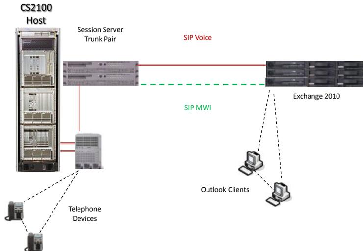
**Figure 1 – Avaya CS 2100 and Microsoft Exchange 2010 UM Setup**
