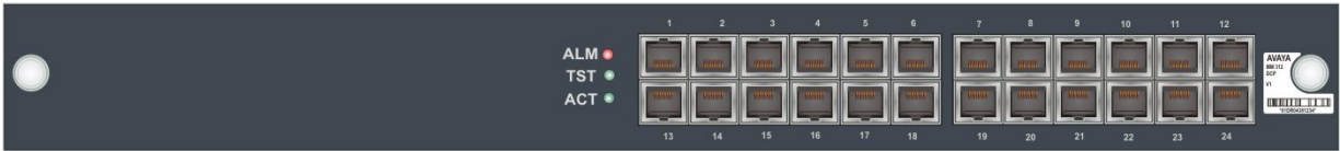
Figure 39: The MM312 media module front panel
