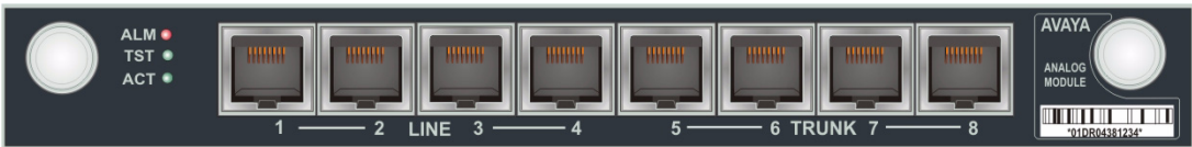
Figure 47: The MM714 media module front panel
