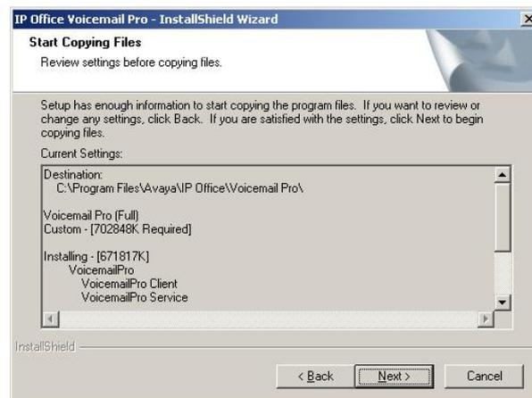
13. The new version of IP Office software will now be installed. PHP will also be installed during this process.
