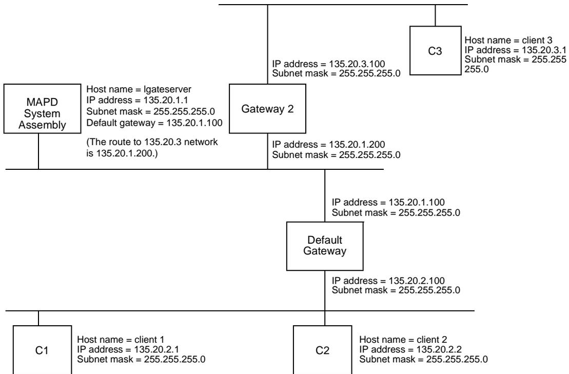
This sample configuration shows the CV/LAN application with different clients on networks physically different from that of the MAPD system assembly. The default gateway leads to clients C1 and C2, and gateway 2 leads to client C3. This sample configuration requires that the CV/LAN application and the clients be administered, as follows:
