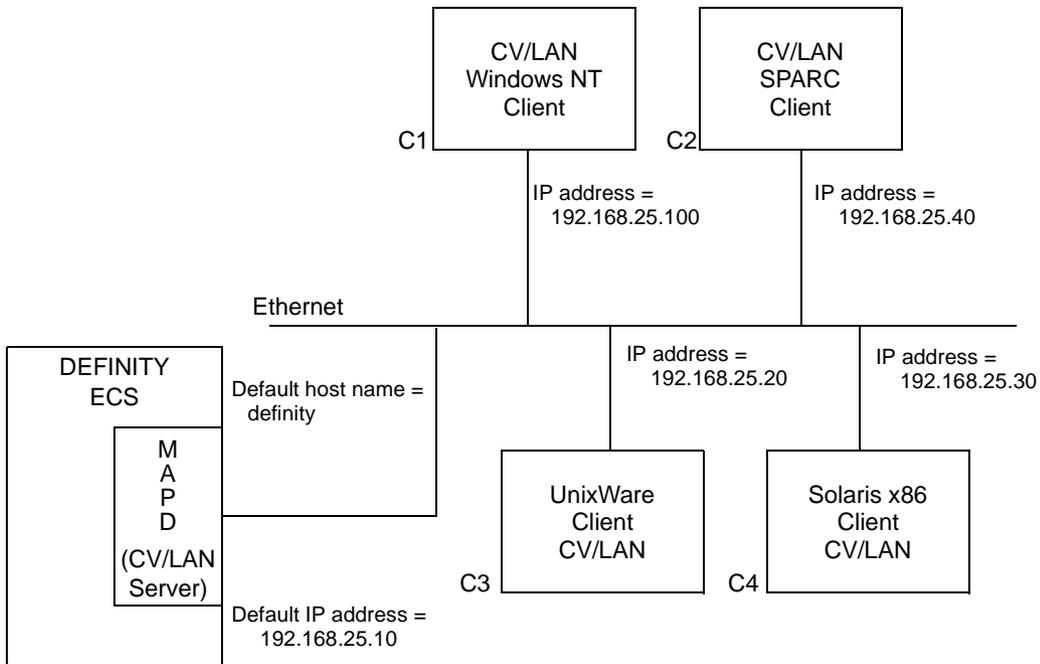
This sample configuration shows the CV/LAN application over MAPD shipped from the factory with defaults already administered (default hostname = *definity* and default IP address = *192.168.25.10*) with the CV/LAN running on the MAPD and four clients, C1, C2, C3, and C4 on the same subnet.
