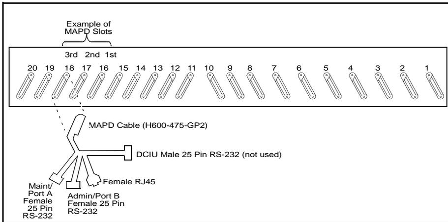
**Figure 2-8. Attaching the MAPD Cable**
