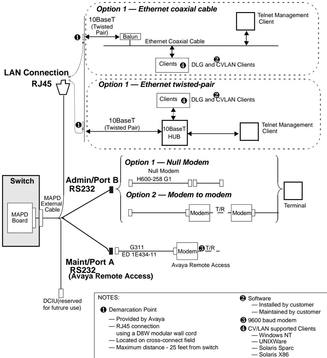
Figure 2-3. MAPD External Cabling and Connection Options
