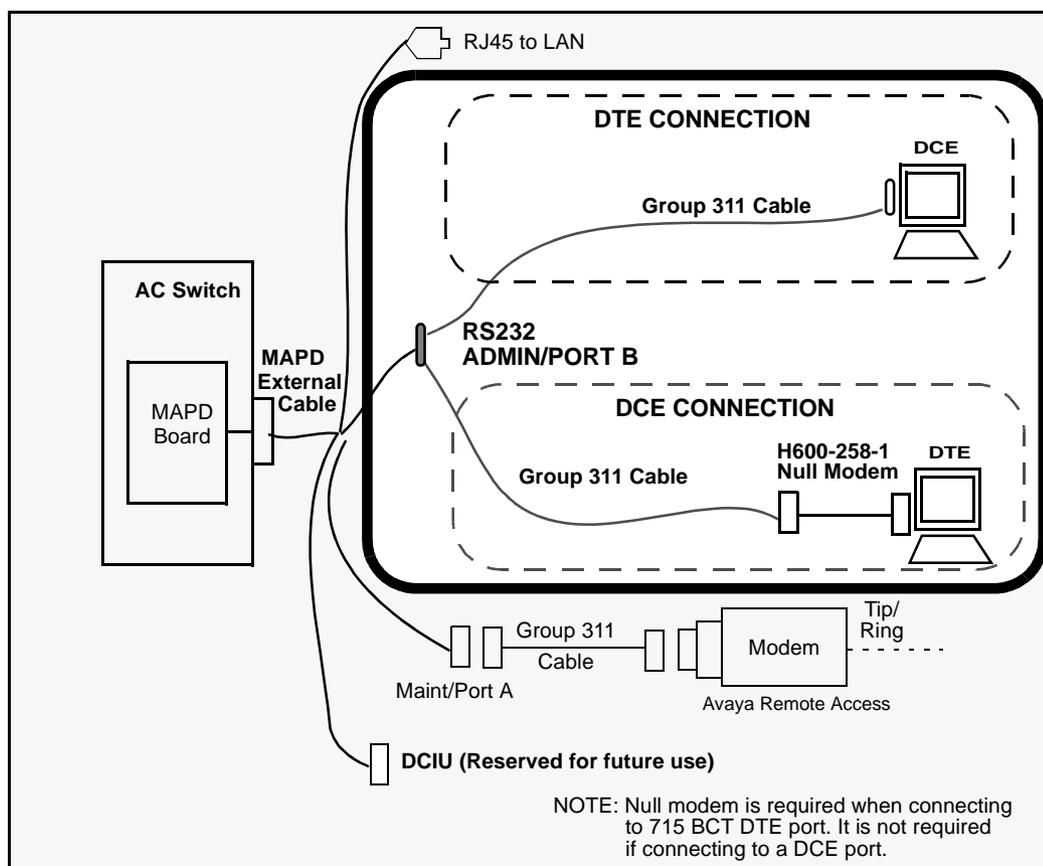
Figure 2-15. Installing a Terminal Via Direct Connection in an AC Switch
