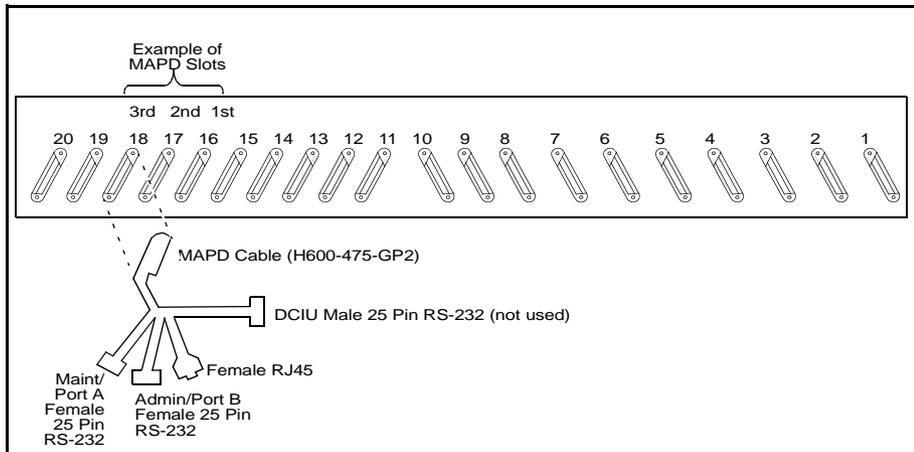
**Figure 2-10. Attaching the MAPD Cable**
