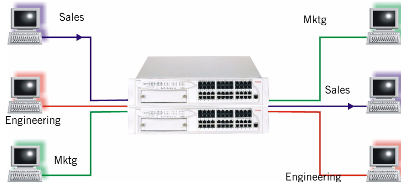
Figure 11.2 VLAN Switching and Bridging
