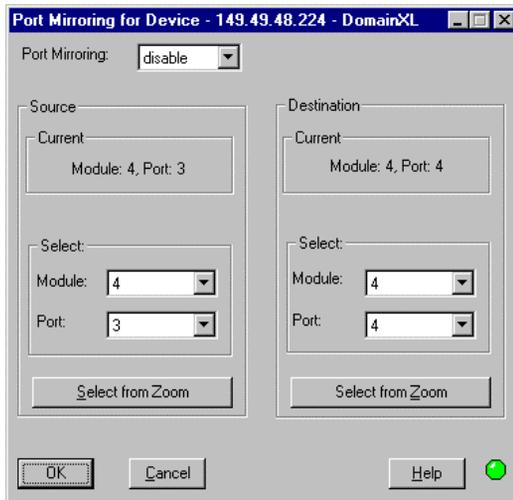
Within the Port Mirroring for Device application, select the Source port (left hand column) and the Destination port numbers (right hand column), from the list of available modules/ports (or from the Zoom selection). Then confirm the configuration by clicking OK.
