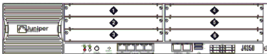
Figure 33: Slot numbers on the Juniper J6350 Services Router
