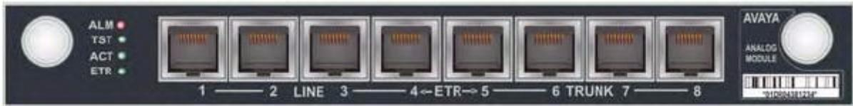
The MM714B analog media module provides all the features provided by the MM714 (see [Standard Media Module LEDs](#)), and in addition provides an emergency transfer relay (ETR). In the event of system failure, the MM714B provides ETR services by connecting trunk port 5 and line port 4.
