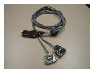
Figure 18: 2-port SDI cable (NTAK19EC) cable
