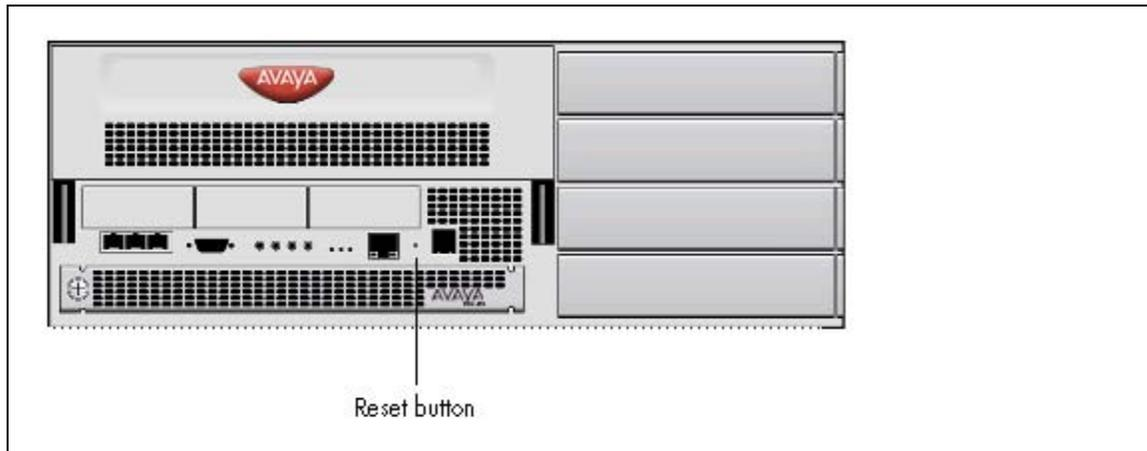
The figure [Reset switch location on BCM50](#) on page 37 shows the location of the reset switch on the BCM50.
