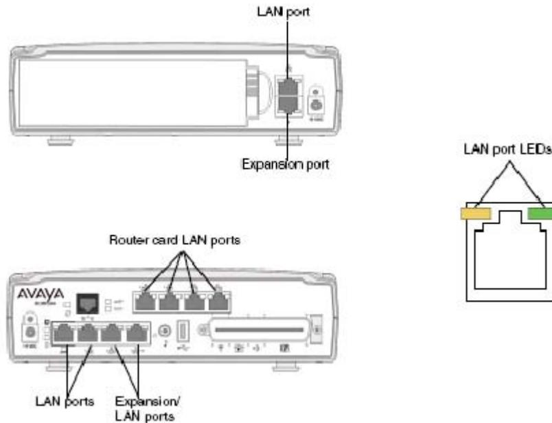
The [LAN port and expansion port LED indicators](#) table describes the possible LED states for the LAN ports LEDs.
