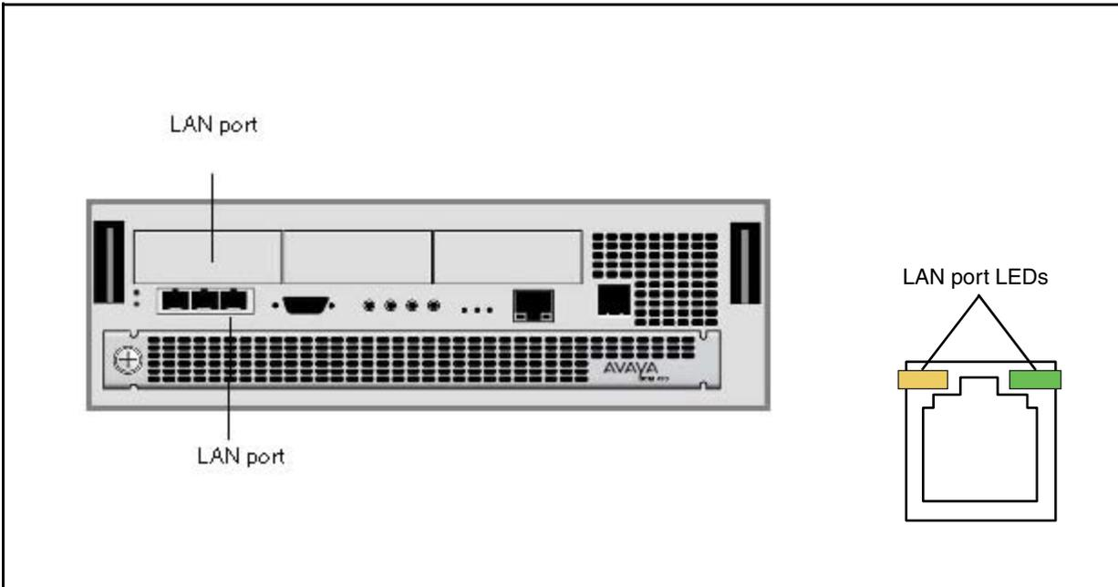
The figure [LAN port LED locations on the Avaya BCM50 main unit](#) on page 21 shows the LAN port LED locations on the Avaya BCM50 main unit. The expansion ports on the BCM50 main unit also function as LAN ports. The expansion port LEDs indicate LAN activity only. The LEDs do not indicate expansion unit presence. The LEDs do not light.
