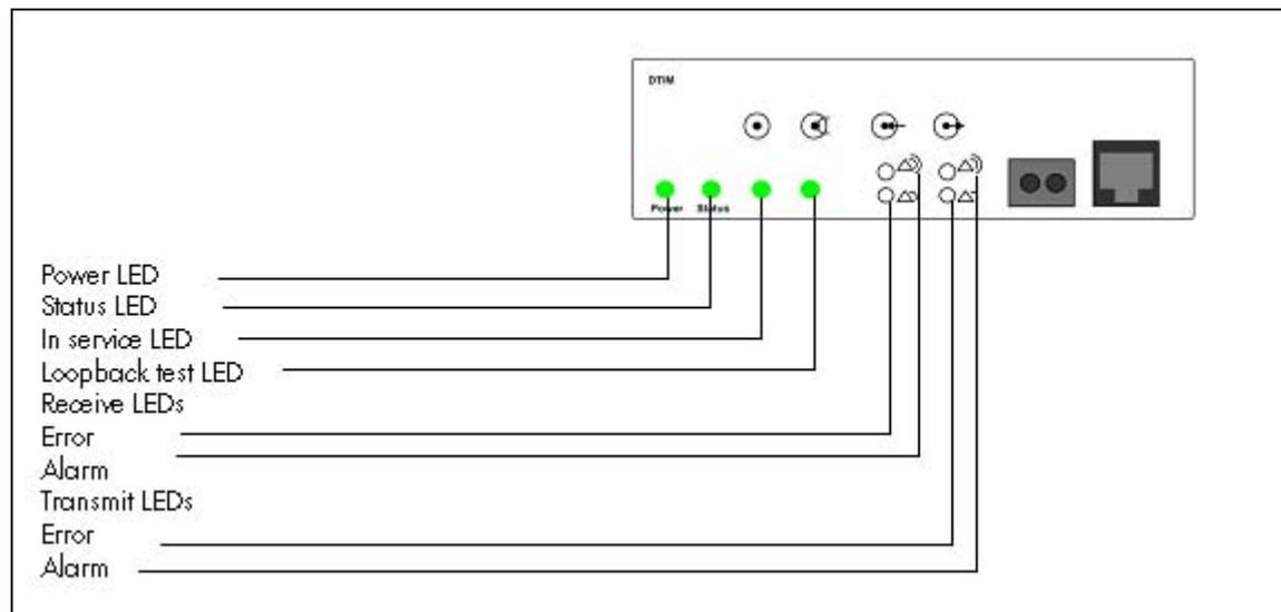
The [DTM LED functions](#) table describes the functions of the DTM LEDs.
