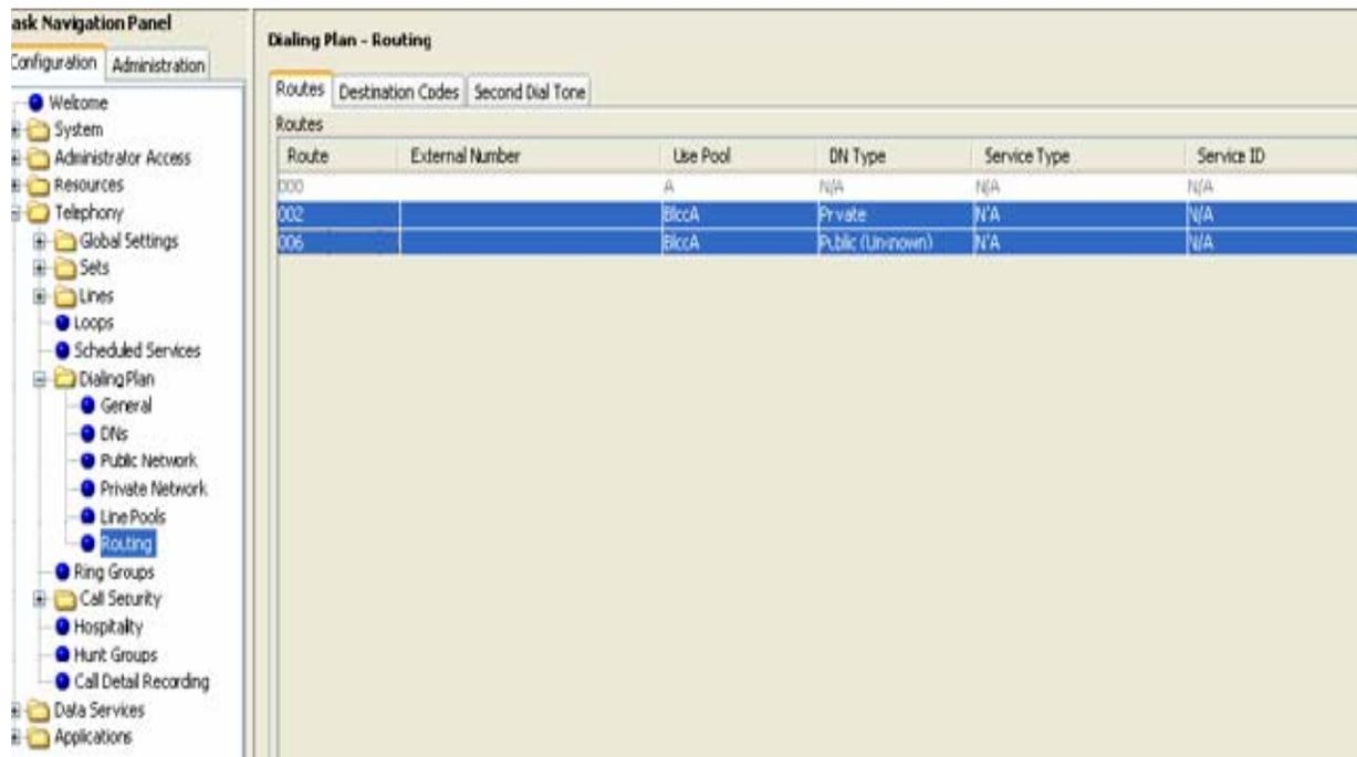
The screenshot shows the Cisco Unified Communications Manager Administration console. The left sidebar is the 'Task Navigation Panel' with 'Configuration' selected. The 'Dialing Plan - Routing' page is active, showing a table of routes. The table has columns for Route, External Number, Use Pool, DN Type, Service Type, and Service ID. Three routes are listed: 000, 002, and 006.
