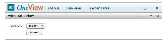
The Wire Data View screen is updated with the located Card LAC entry. Set the Card Type, Wired For, and Wire Group parameters as shown below.
