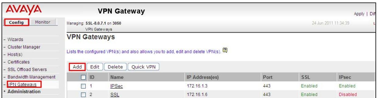
The **VPN Name** was **SSL**. The SSL VPN Portal **IP Address** was set to **172.16.1.6**. This is the IP Address the remote user will use to access the SSL VPN tunnel. The default **Port** number was **443**. The **SSL Status** was **enabled**. The **Create VPN** button was selected to save the changes.
