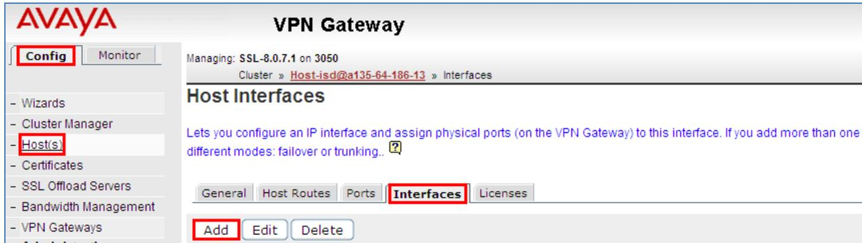
Interface One had **IP address** set to **135.64.186.13**, the inside interface. The **Netmask** was set to **255.255.255.224** and the **Default Gateway** was **135.64.186.1**. Interface **1** was **Selected** from the **Port(s)** column. The **Update** button was selected to update the configuration.
