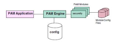
The PAM application interacts with the PAM engine through a PAM conversation. When the PAM application needs to process a new login session, it calls the PAM engine to begin the conversation. The PAM engine then scans the configuration files to check the specified login mechanism. A PAM configuration file consists of the following four sections:
