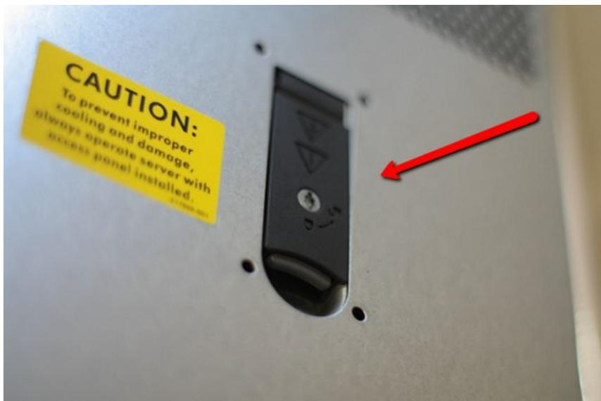
3. Turn the screw to the 'unlock' position.
