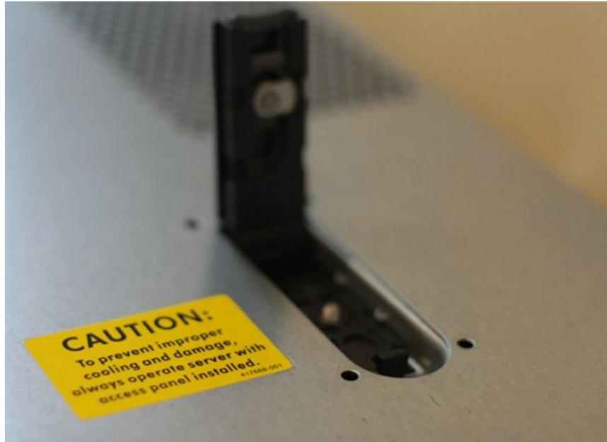
5. Lift up the cover to remove it and then locate the internal USB port.
