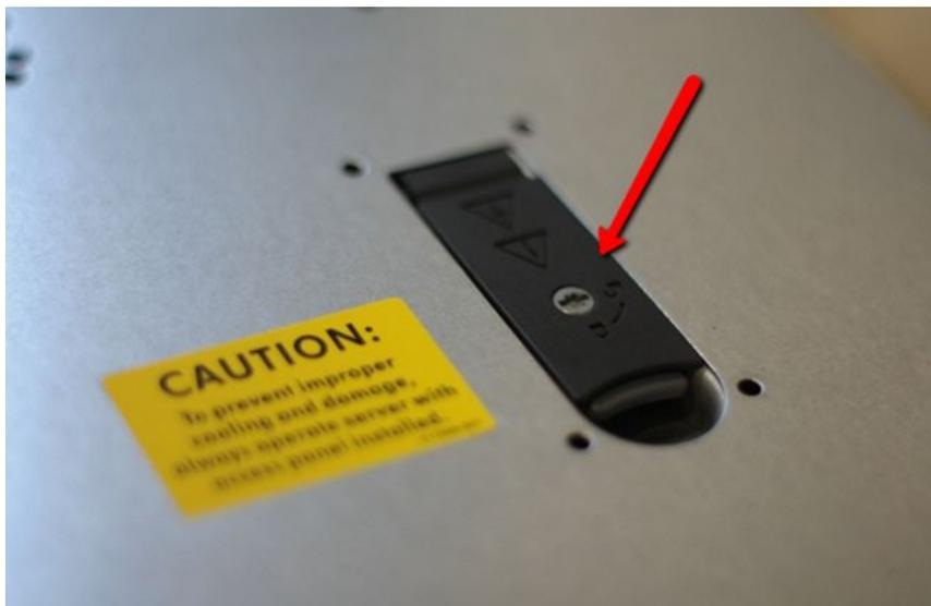
4. Gently pull the lever all the way upward to open the cover of the server.
