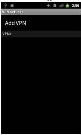
3. Select Add VPN, Add L2TP/IPSec PSK VPN to configure a pre-shared key based L2TP/IPSec VPN.
