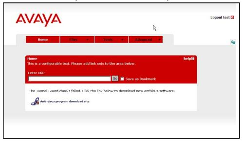
To confirm that Avaya Endpoint Access Control Agent is running but the checks have failed, the Avaya Endpoint Access Control Agent Failure icon is displayed to the right of the Portal tabs (for an explanation of the other icons, see Chapter 6, "The Portal from an End-User Perspective").
