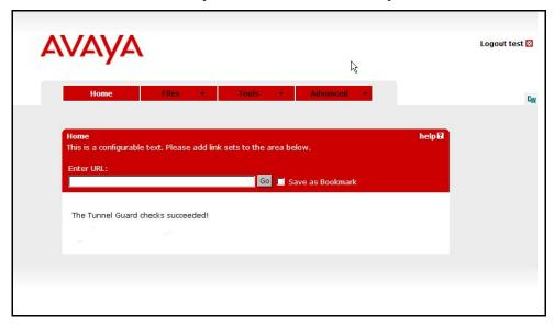
To confirm that Avaya Endpoint Access Control Agent is running and that the checks have succeeded, the Avaya Endpoint Access Control Agent Success icon is displayed to the right of the Portal tabs (for an explanation of the other icons, see Chapter 6, "The Portal from an End-User Perspective").
