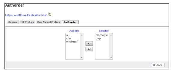
**NOTE** – You must configure MSCHAPv1, CHAP or PAP as primary authentication for L2TP with Apple or Android clients. MS-CHAPv2 does not work for L2TP with Apple and Android clients.
