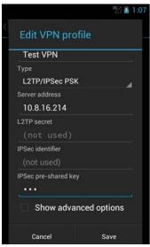
5. Configure the VPN Type as L2TP/IPSec PSK.
