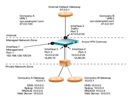
Figure 17-1 Two VPNs on a Single AVG Platform
