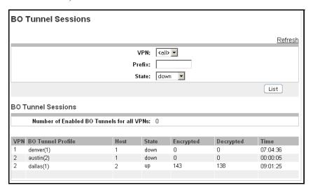
The output shows the name of the branch office tunnel profile, the Avaya VPN Gateway host from which the tunnel is set up, the tunnel state (up, phasel or down), encrypted data in kBytes and decrypted data in kBytes. The up tunnel state means that both ISAKMP and IPsec SAs are established, whereas the phasel state indicates that only the ISAKMP SA is established).
