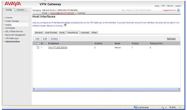
Verify that the management interface on the "private" or "internal" side of the Avaya VPN Gateway has the correct IP address and network mask. Also verify that this interface uses the desired physical port on the Avaya VPN Gateway (displayed under Port(s).
