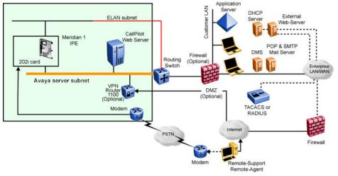
The following figure shows an example of a network in which an Avaya CallPilot server is connected to an Avaya Communication Server 1000 switch (AML connectivity).
