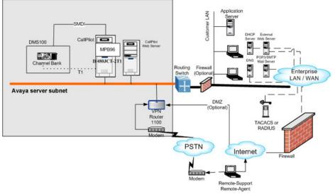
The following figure shows an example of a network in which a CallPilot server is connected to an SL-100<sup>\*</sup> switch (T1/SMDI connectivity).
