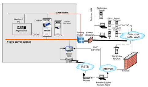
The following figure shows an example of a network in which a 202i server is integrated into an Avaya Communication Server 1000 switch
