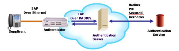
Figure 39: 802.1x and EAP network architecture
