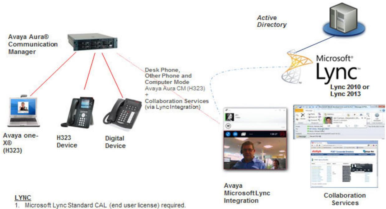
Figure 1: Lync Integration deployed in an Enterprise with an H.323 endpoint
