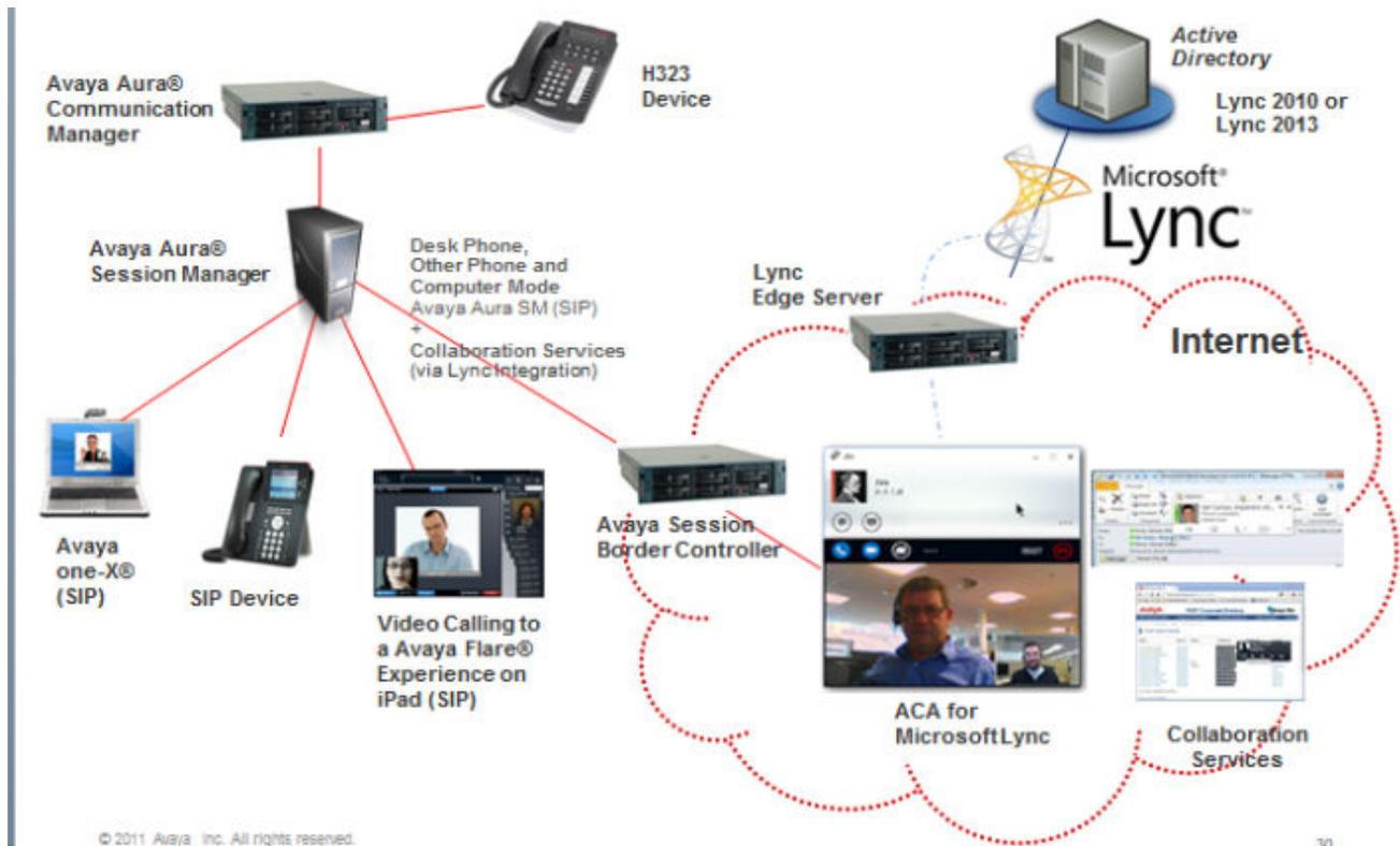
Figure 4: Lync Integration with a SIP client in an Internet deployment
