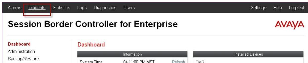
Use the Incident Viewer to verify Server Heartbeat and to troubleshoot routing failures. This verification is applicable if the Trunk server supports Heartbeat mechanism and is configured in the deployment.
