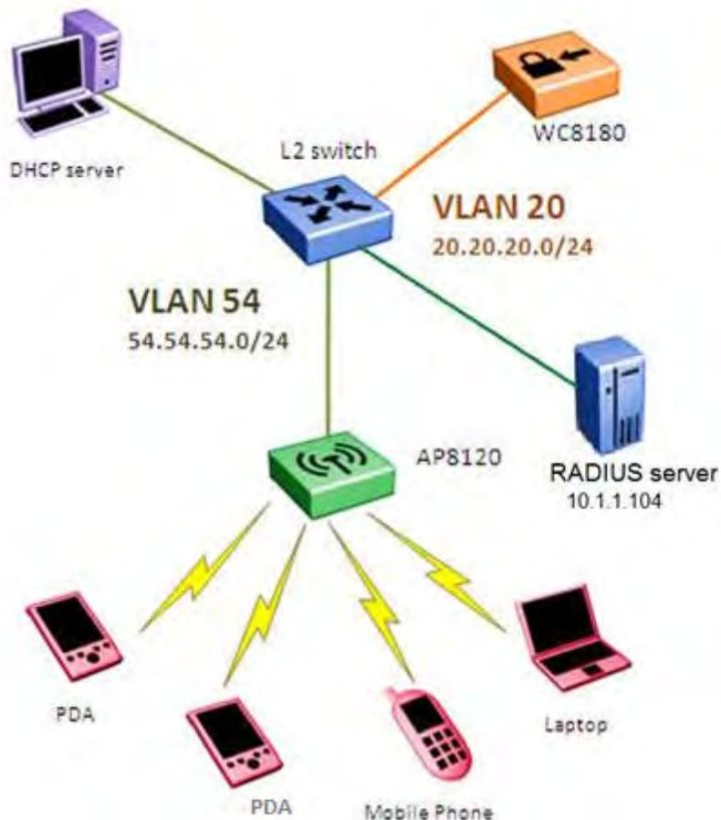
Figure 1: WLAN 8100 Overlay network design example
