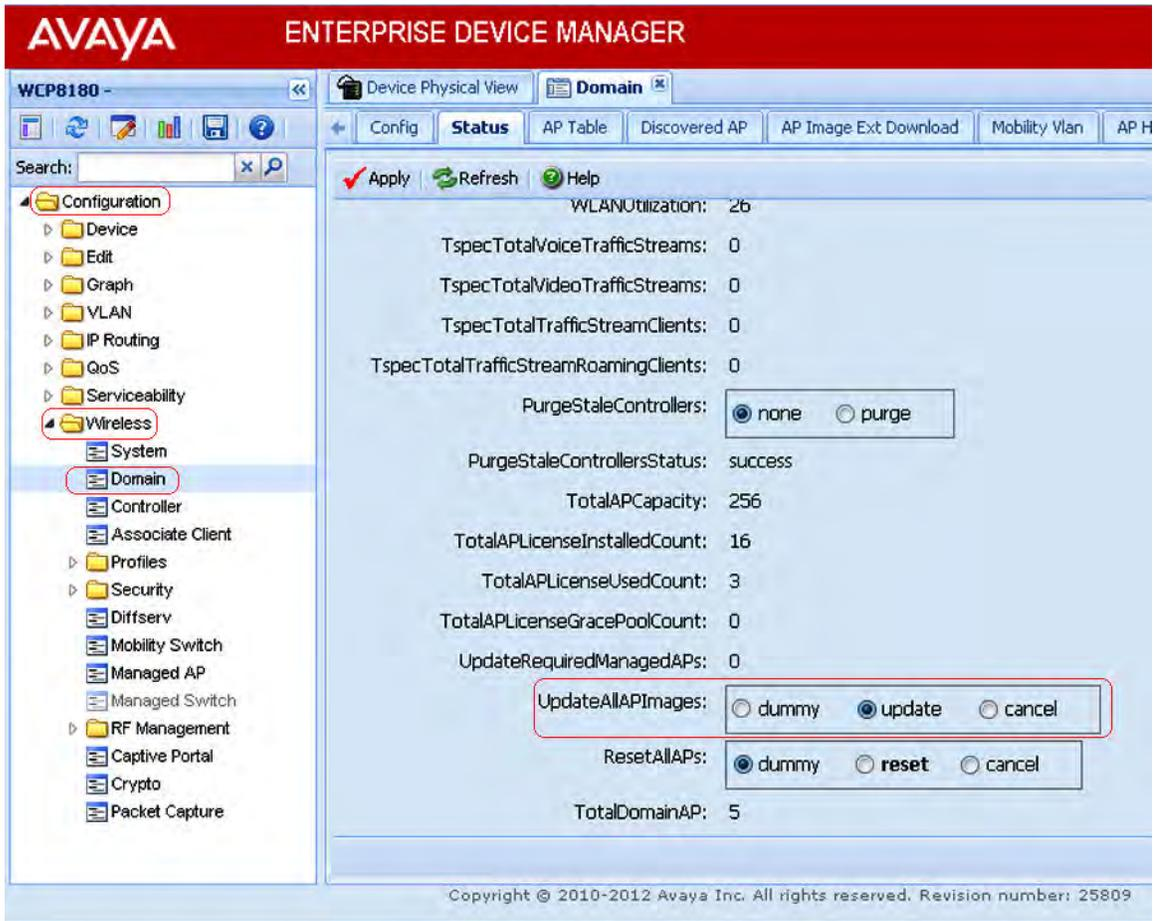
12. Complete the following steps to create profiles (network, radio and AP profiles) using the EDM. These steps are provided for demonstration purposes.
