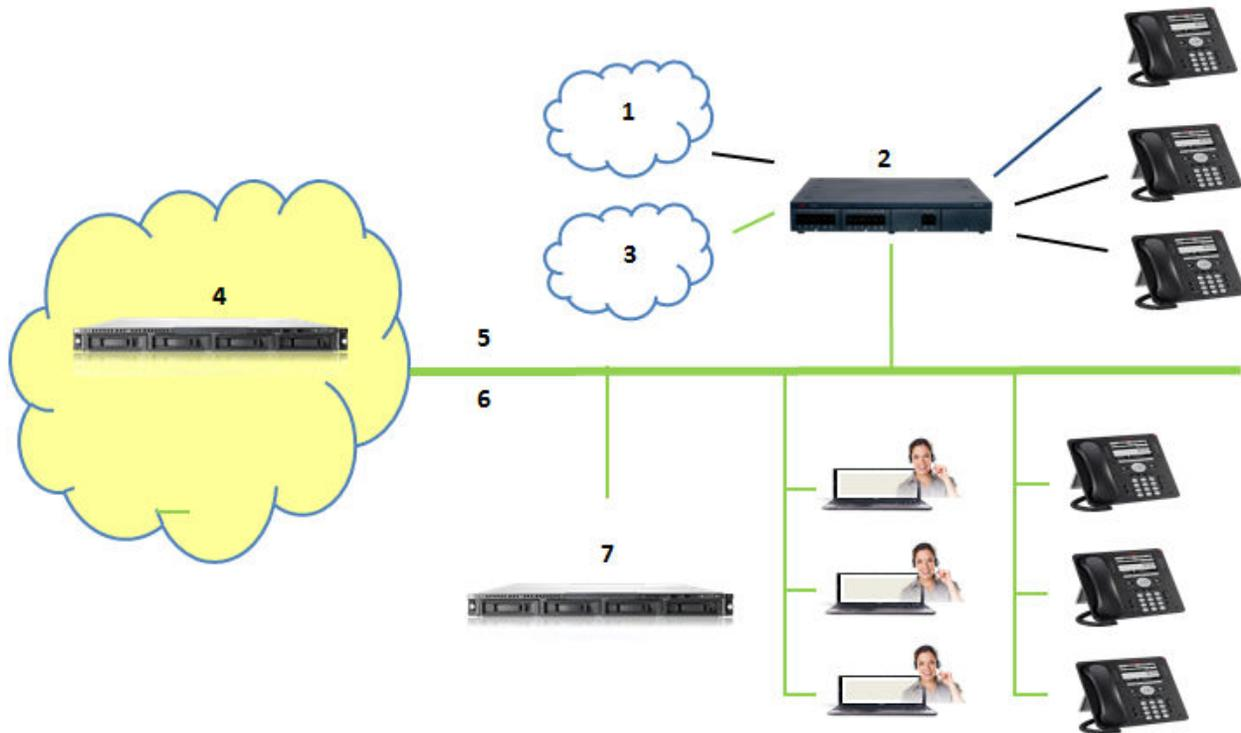
**Figure 23: IP Office Contact Center cloud topology**
