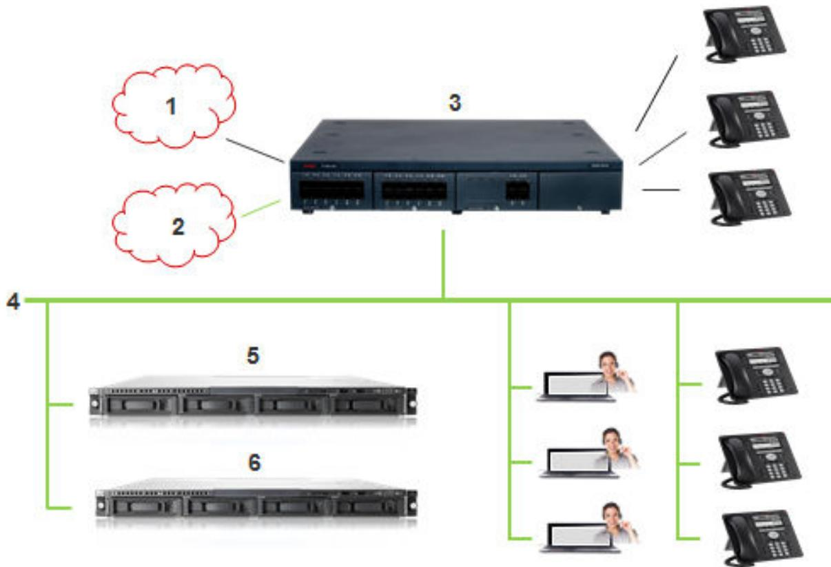
Figure 22: IP Office Contact Center IP500 V2 topology
