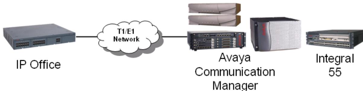
**Figure 28: Q.SIG networking using T1/E1 links (TDM)**
