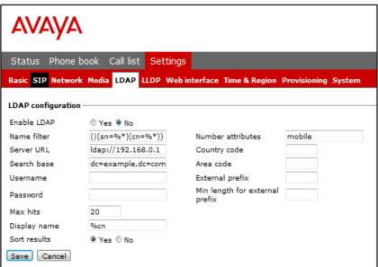
Avaya B179 has support for an external phone book, which means it can communicate with a directory server using LDAP (Lightweight Directory Access Protocol). The built in search function dynamically filters the content from the LDAP database, based on the search characters the user enter.
