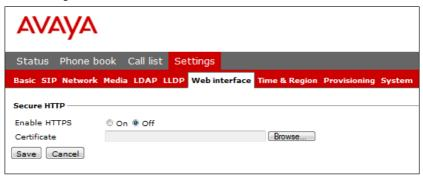
The web server in the Avaya B179 supports secure connections using HTTPS.
