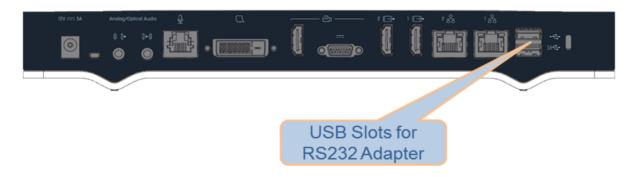
If you are using a serial port, you must use the same baud rate configured in XT system, which by default it is **115200**. Moreover the system can be configured to avoid the need to send the AT initialization command.
