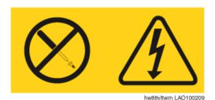
Hazardous voltage, current, and energy levels are present inside any component that has this label attached. These components do not contain any serviceable parts. If you suspect a problem with one of these parts, replace the power supply.
