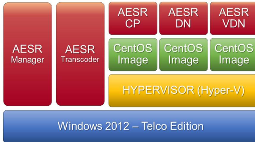
Figure 2: Components in an All-In-One Deployment with Virtual Software
