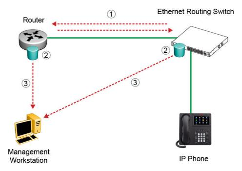
Figure 6: How LLDP works
