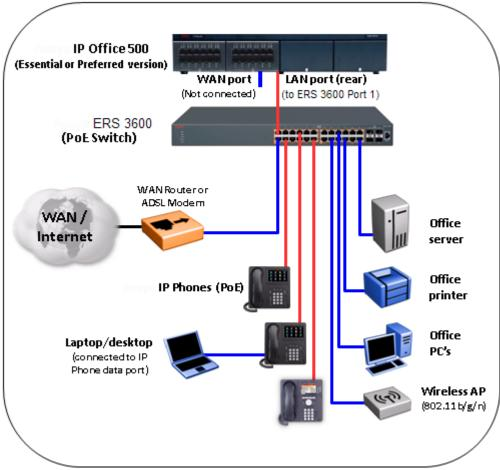
Figure 8: IP Office physical solution reference diagram
