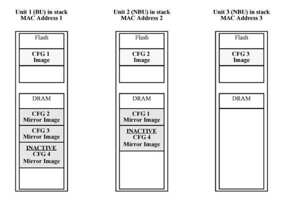
Figure 3: CFG mirror images after removing unit 4
