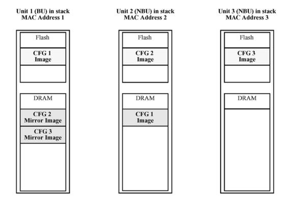
Figure 1: CFG mirror process in stack
