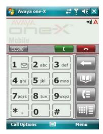
There are two main screens—the Dial Pad screen and the Calls View screen. The Dial Pad screen provides a more convenient way to enter digits, rather than using the Pocket PC keyboard. The Calls View screen shows the phone number and call timer for your active calls. Select [[11]] (the Dial Pad/Calls View soft button) to toggle between the two screens.
