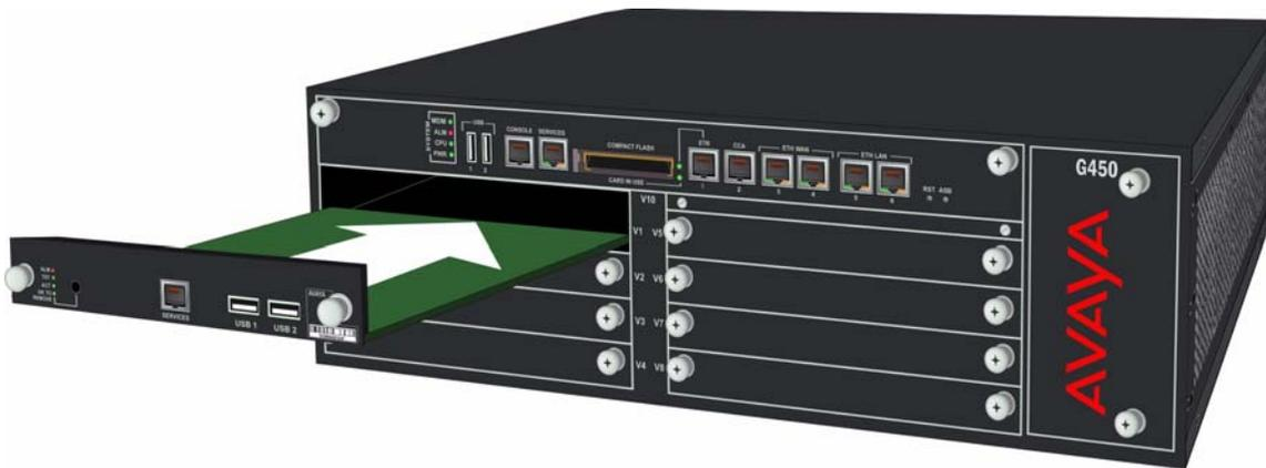
5. Apply firm pressure to engage the connectors.
