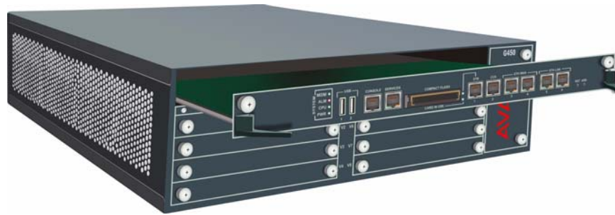
Figure 8: Removing and inserting the G450 main board
