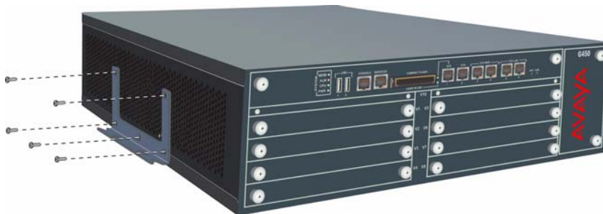
Figure 4: Wall mounting bracket placement
