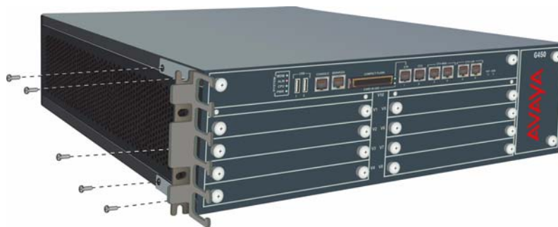
Figure 3: Attaching a mounting bracket with cable guides
