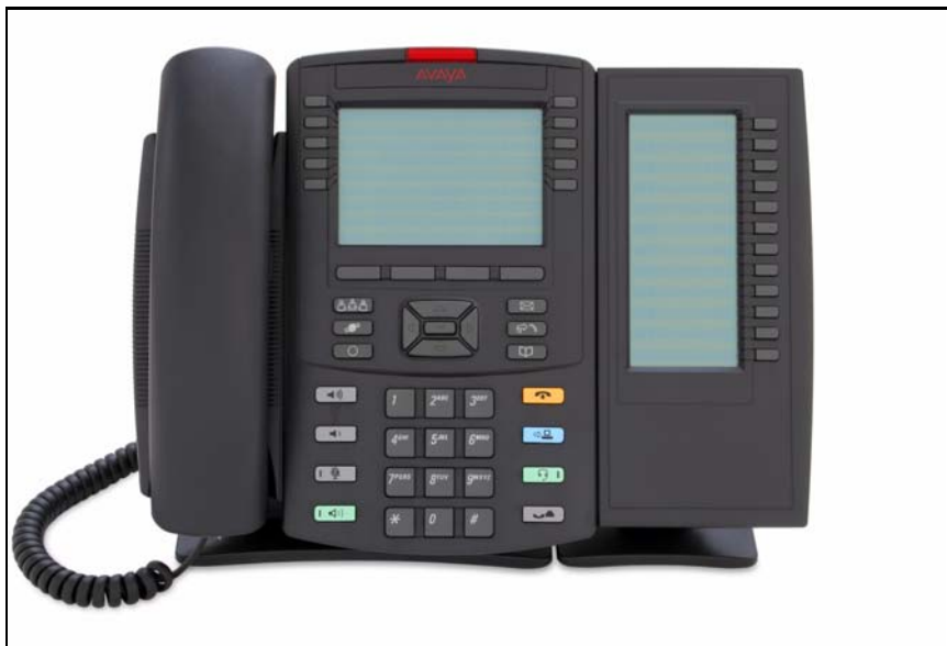
Figure 1: Avaya 1230 IP Deskphone with the LCD Expansion Module: 12-key Self labeling
