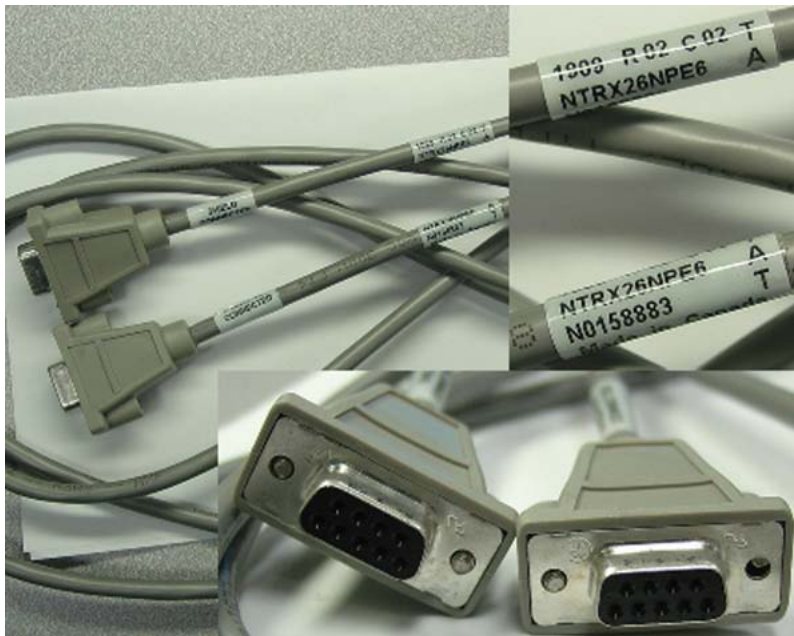
Figure 180: NTRX26NPE6 9 pin female to 9 pin female null modem cable
