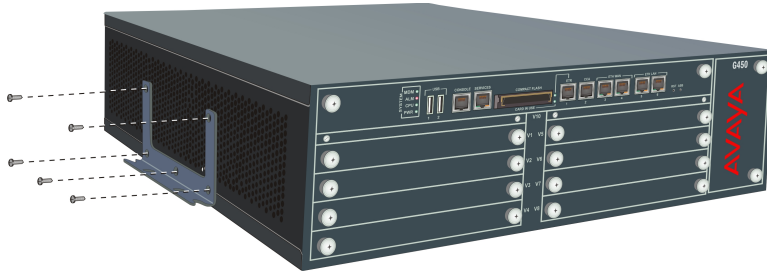
Figure 1: Attaching a bracket to each side of the Branch Gateway
