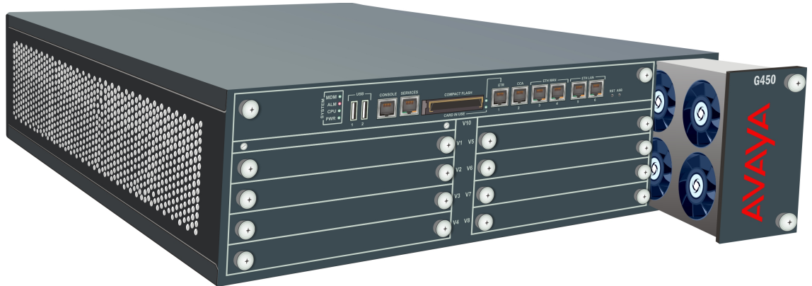
Figure 35: Replacing the fan tray
