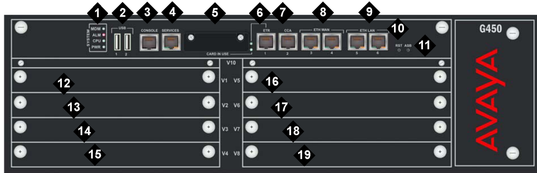
Figure 39: The G450 1.x front panel ports and slots
