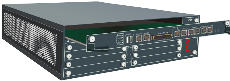
Figure 26: Removing and inserting the Branch Gateway main board
