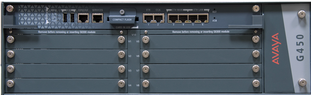
Figure 40: The G450 2.x front panel ports and slots
