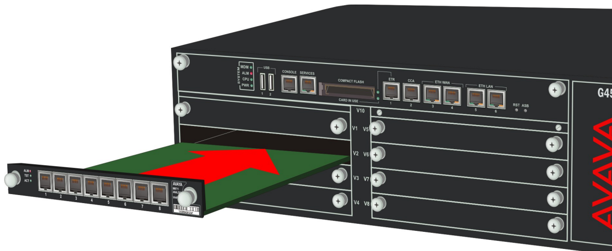
Figure 5: Inserting a media module
